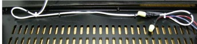
5. Attach connectors from harness to back of the LED light in top panel.
